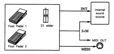
**Assign** Assign CC0 - CC95/AFTERTOUCH/BEND-UP/BEND-DOWN/PROG-UP/PROG-DOWN These settings determine the parameters which will be controlled by the pedal or C1 slider. CC0-CC95 are control change numbers 0 - 95. BEND - UP / BEND - DOWN indicates pitch bend up and down. PROG - UP / PROG - DOWN will select the next higher or lower Performance or Patch. The value in parentheses ( ) indicates the current position of the pedal or C1 slider.
