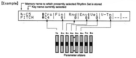
The values from the left correspond to parameter sliders 1 - 8. Move the appropriate parameter slider to modify the desired value.
