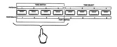
\* The on/off setting you make for each Tone using the TONE SWITCH buttons ([1]---[4]) is stored as part of the Patch settings when you use the Write operation (p.87).
