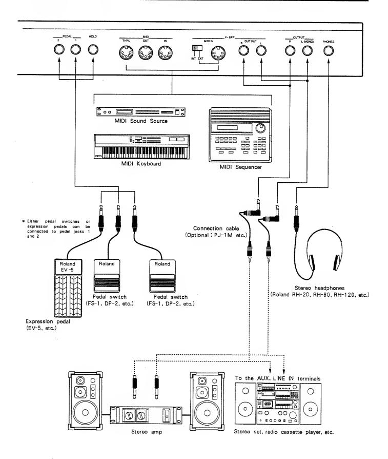
Connect the MIX(INT) OUT jack on the rear of the JV - 90 to an amplifier/speaker setup (stereo set). You can also connect stereo headphones to the PHONES jack.
