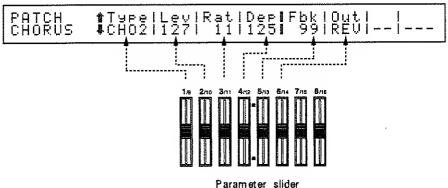
The values from left to right correspond to parameter sliders 1-8. Move the parameter slider (or [DEC]/[INC]) corresponding to the parameter you wish to modify (p.6).
