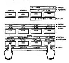
If you press the buttons only for a short time (less than one second), the internal sound source will be muted, and Key Off / Hold Off messages will be transmitted to each channel for which there is a Key On / Hold On. If you press the buttons for more than one second, the following messages will be transmitted to all channels.
