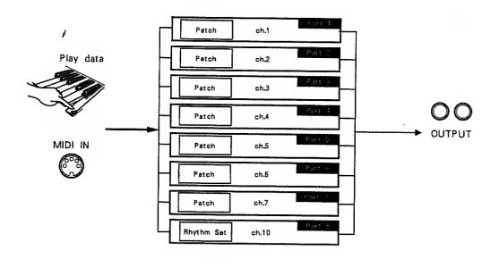
As shown in the figure above, one Patcb is assigned to each Part of the ensemble Performance. By changing Patches, you can make an ensemble Performance with the ideal sounds for each Part.
