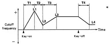
For nagative (-) values of Envelope Depth, the polarity (+/-) of the cutoff frequency change will be inverted.
